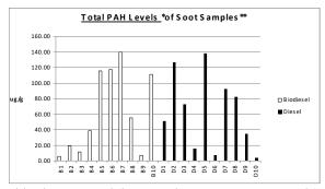
\* Total PAH Level (in ug total PAH per g soot sample) \*\* B1 to B10 are biodiesel samples, D1 to D10 are diesel samples
