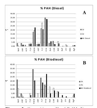
**Figure 3.** Composition profile of PAH (% or g individual PAH/100 g total PAH) in particulate matter from exhaust of three diesel-fueled vehicles: 1d and 2d are tailpipe soot samples, MJ Diesel is a filter particulate sample (A); 1b and 2b are tailpipe soot samples, MJ Biodiesel is a filter particulate sample (B). The abbreviated PAH labels in the axis are fully spelled out in Figure 2.
