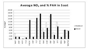
% PAH: g individual PAH per 100 g total PAH (average of 10 samples from different vehicles per fuel category) \*<u>except</u> for NO<sub>2</sub> (calculated as 10\* [uL gas per mL absorbing solution])
