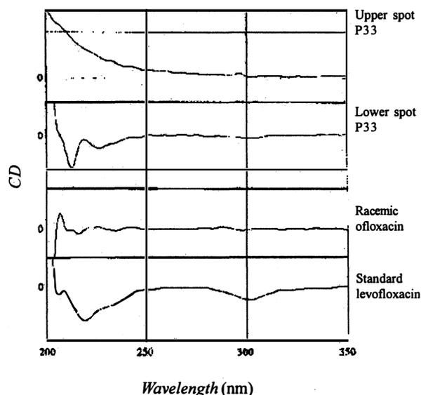
Fig. 3. CD-ORD spectra for levofloxacin and ofloxacin compared with that obtained from upper and lower spots of P33 TLC plate. Conditions: Range- 350 to 200 nm; Bandwidth – 2.0 nm; Sensitivity – 100 mdeg; Resolution – 0.5 nm; Response – 1 sec; Speed -100 nm/min; Accumulation-1.
