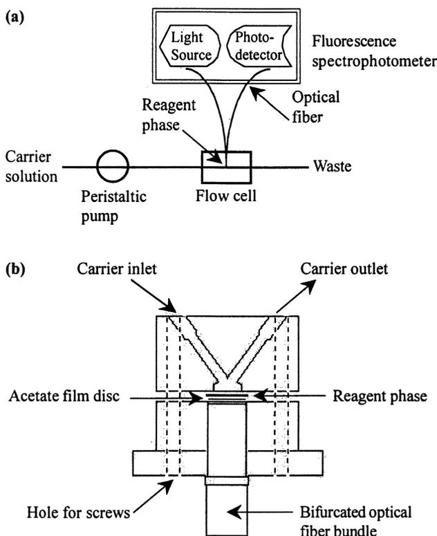
Fig. 1. (a) Instrumentation system based on a fluorescence spectrophotometer; (b) Diagram of flow-cell
