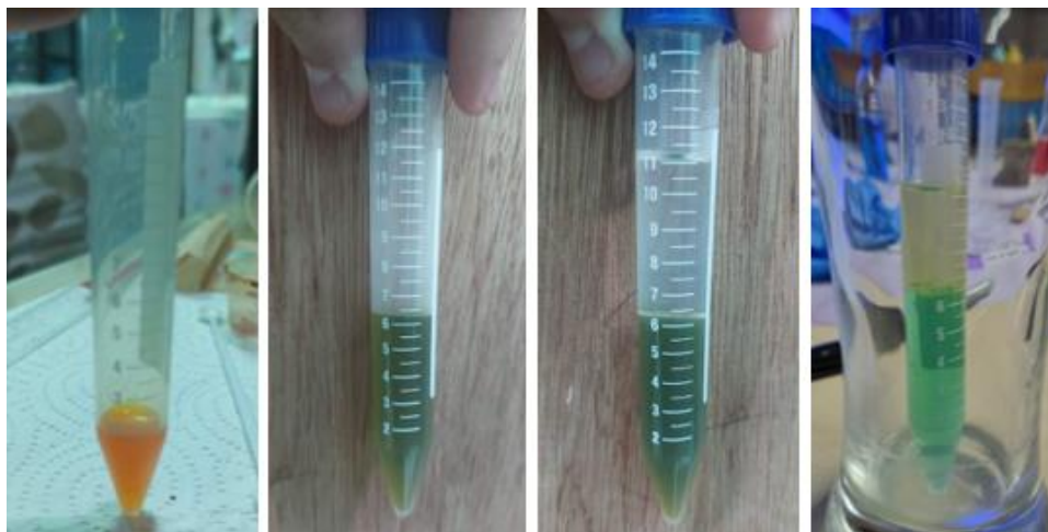
Figure 3. Progression photos of the extraction of spices experiment, illustrating the transfer of the yellow pigments to the nonpolar oil layer
