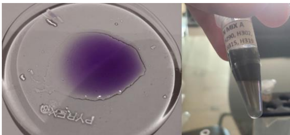
Figure 5. (Left) Results for the Ninhydrin test of MSG; (Right) Result for the Tollens' test of glucose.
