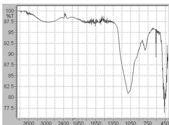
**Figure 2B.** FTIR of Phen-Si.
