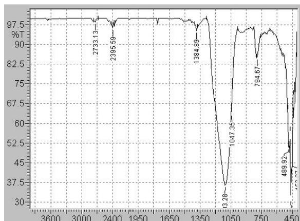
**Figure 2A.** FTIR of silylated silica.
