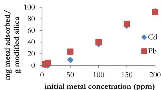
**Figure 4.** Cd and Pb Adsorption (Equilibrium Method)
