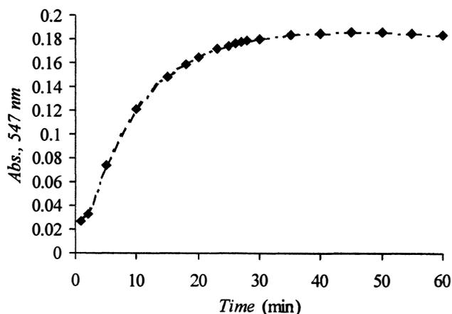
Fig. 2. Optimum reaction time for 100 µg/L BrO<sub>3</sub><sup>-</sup> and 19 ppm fuchsin reagent.
