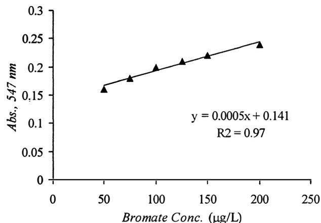
Fig. 4. Low BrO<sub>3</sub><sup>-</sup> concentration calibration curve.
