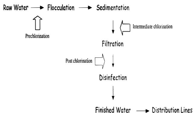
Fig. 1. Basic processes in water treatment.
