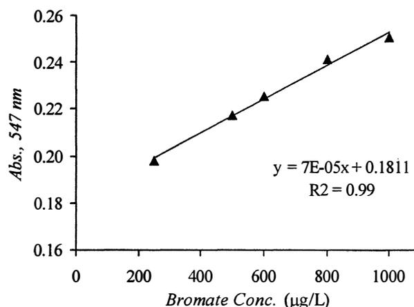
Fig. 5. High BrO<sub>3</sub><sup>-</sup> concentration calibration curve.
