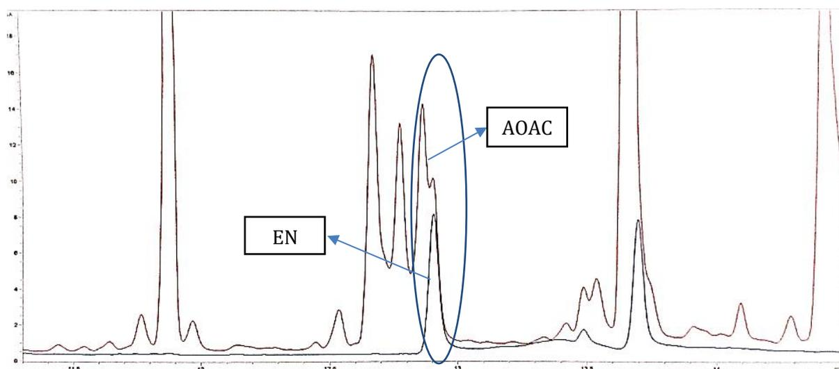
Figure 1. GC-NPD chromatogram using QuEChERS AOAC and EN methods
