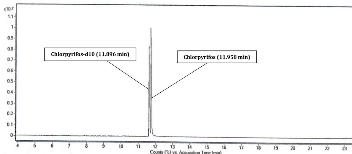
Figure 2. GC-IDMS/MS chromatogram of chlorpyrifos at and chlopyrifos-d10
