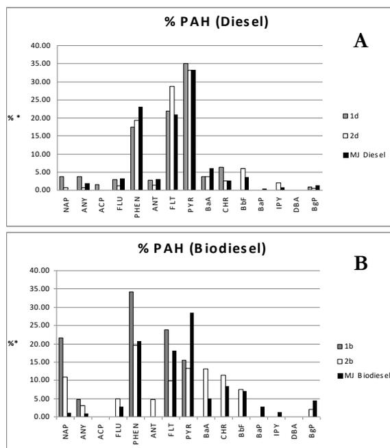
**Figure 3.** Composition profile of PAH (% or g individual PAH/100 g total PAH) in particulate matter from exhaust of three diesel-fueled vehicles: 1d and 2d are tailpipe soot samples, MJ Diesel is a filter particulate sample (A); 1b and 2b are tailpipe soot samples, MJ Biodiesel is a filter particulate sample (B). The abbreviated PAH labels in the axis are fully spelled out in Figure 2.
