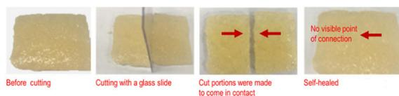
Figure 4. Illustration of the Self-healing Assay Used for the Hydrogels.
